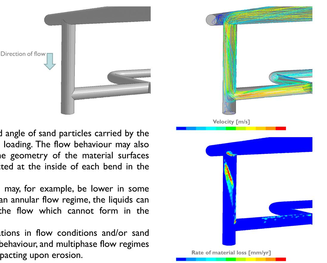
It is important to recognise that the rate of material loss is likely to vary, both in magnitude and the location of any erosion hotspots, during the operational life. This may be due to
